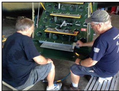
Al Herum and Johnny Schauer fabricating a new lower step on Lil's entrance door.
